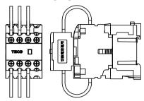
\*主迴路導線安裝在電磁接觸器本體上,切勿安裝於頂裝式接點組。 The main circuit wire is installed on the electrical contactor body, do not installit one the top-mounted contact group.
