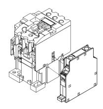
) 將CNA-111SR 門與CU-9~40R 扣緊 . The latch of CNA−111SR fasten with CU−9∼40R.
